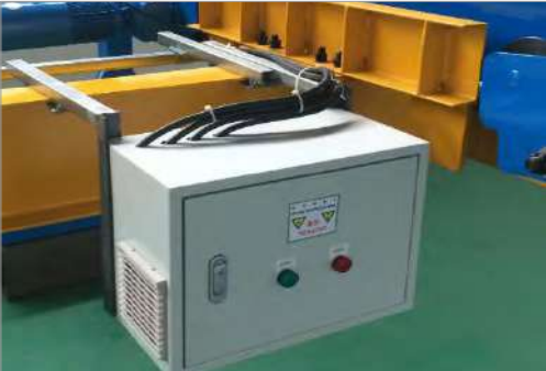
电控箱 Electric control panel
