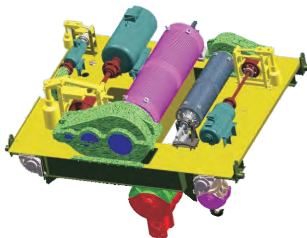
Double girder overhead crane traversing trolley
