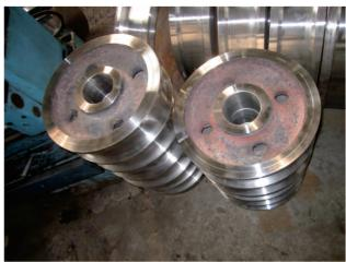
To realize the rough machining of the outer and inner contour surface of wheel blank, and clean up the spare parts of the blank quickly.
