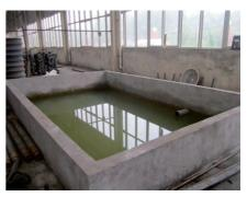
Quenching and tempering is widely used as our heat treating capabilities. It is designed for maximum flexibility by allowing us to heat treat a wide variety of materials, diameters, thicknesses and bore sizes. We are now able to provide virtually any heat treatment for carbon and alloy steels. This quench and temper facility is most applicable to gear blanks, rollers and miscellaneous forgings in specialty applications.
