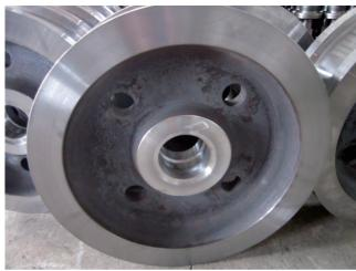
Forged Steel Crane Wheels are available in a wide range of standard sizes. In addition, crane wheels to meet your special design requirements can be produced in virtually any size, configuration and surface finish condition. We maintain a large inventory of carbon and alloy steels to meet your specific needs.
