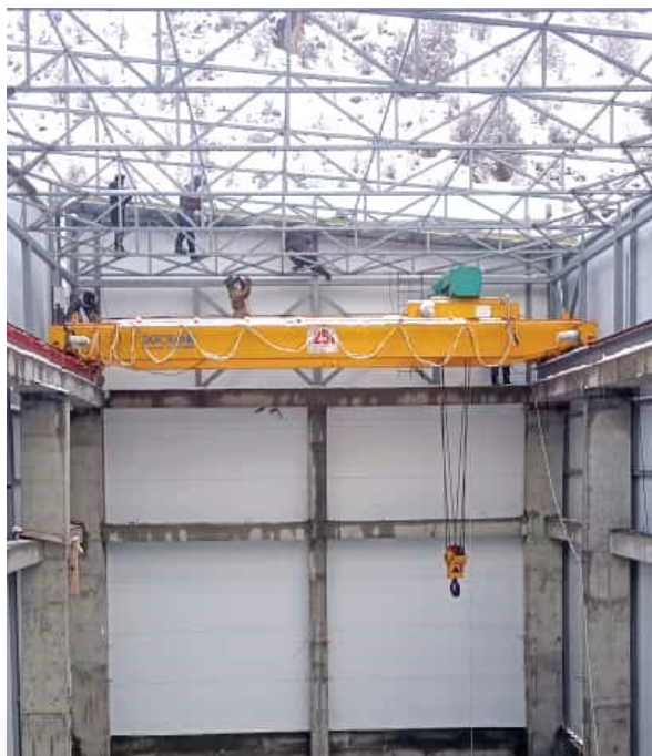
▲ LH25t Double Girder Overhead Crane in TKyrgyzstan
