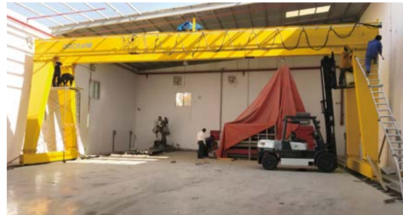
▲ MG10t Double Girder Gantry Crane in Saudi Arabia
