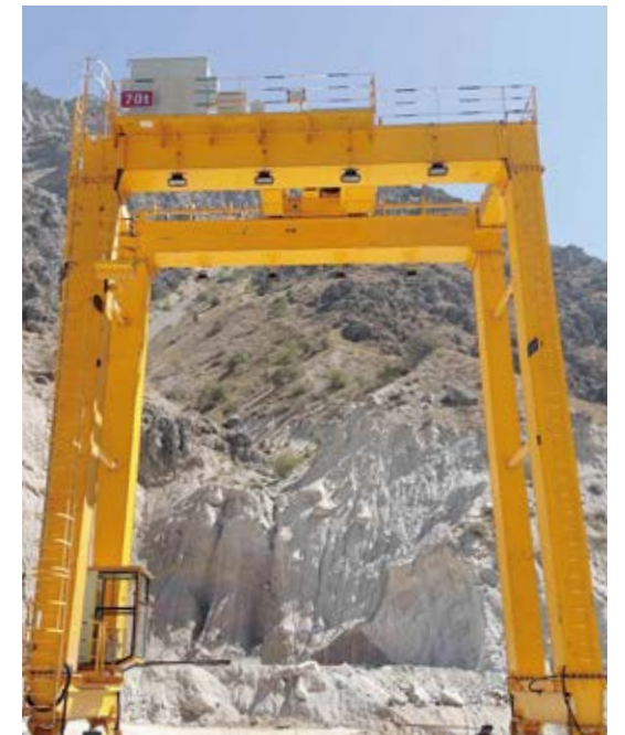
▲ MG70t Double Girder Gantry Crane in Uzbeksitan
