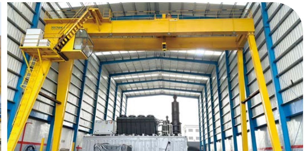
▲ MG40t Double Girder Gantry Crane in Nigeria
