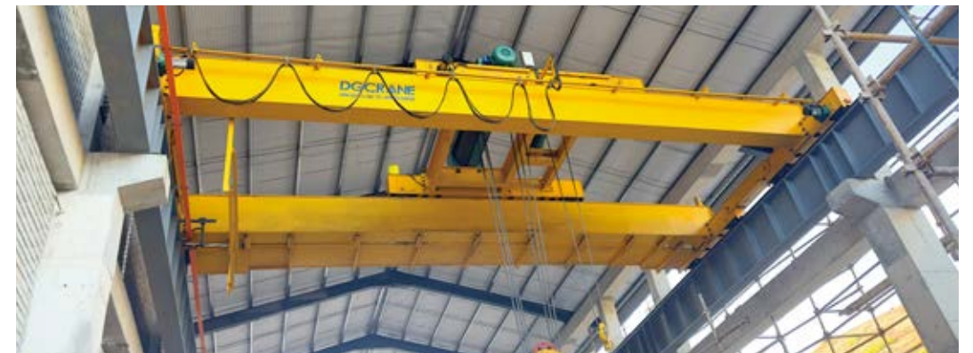
▲ LH25/5t Double Overhead Crane in Zimbabwe
