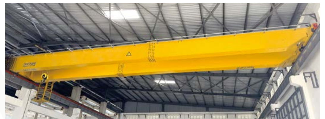
▲ NLH16t Double Girder Overhead Crane in Tanzania
