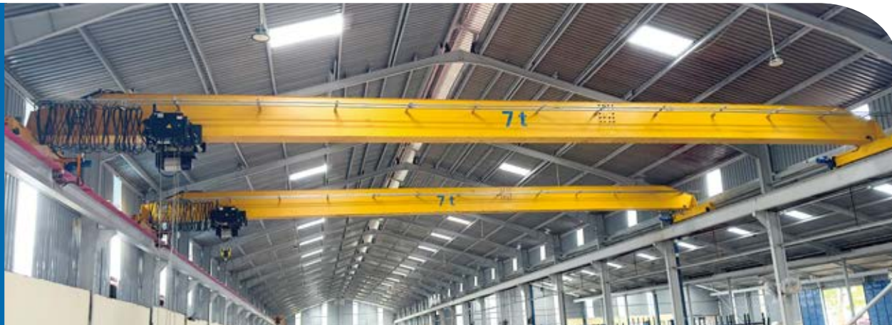
▲ HD7t Single Girder Overhead Crane in Tanzania
