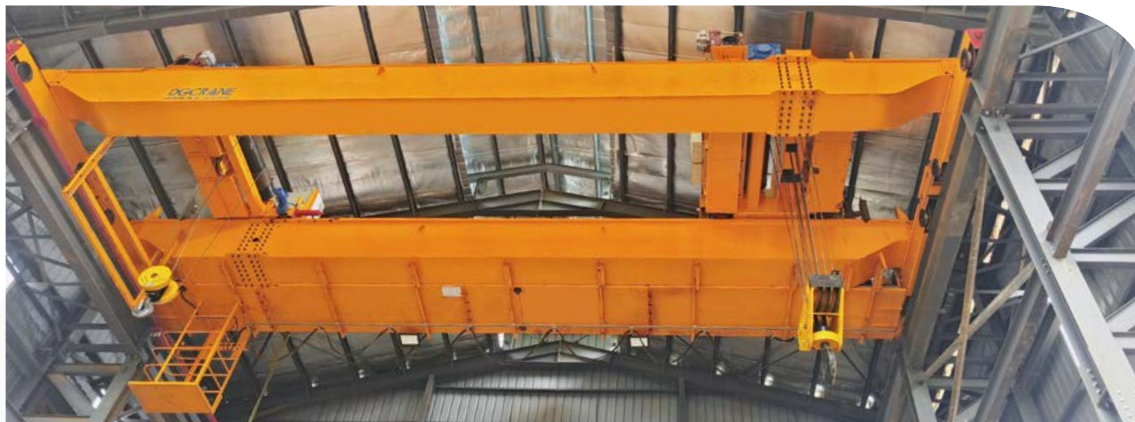
▲ QE40+15t Double Girder Overhead Crane in Tanzania (for Hydropower station)
