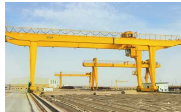
▲ MGE5+5t Double Girder Gantry Crane in Saudi Arabia
