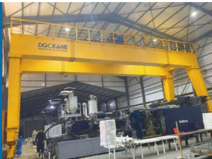
▲ MG100t Double Girder Gantry Crane in Algeria
