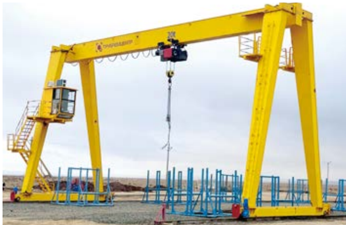
▲ MH20t Single Girder Gantry Crane in Kazakhstan
