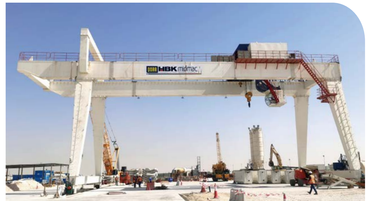
▲ MG60/5t Double Girder Gantry Crane in Qatar
