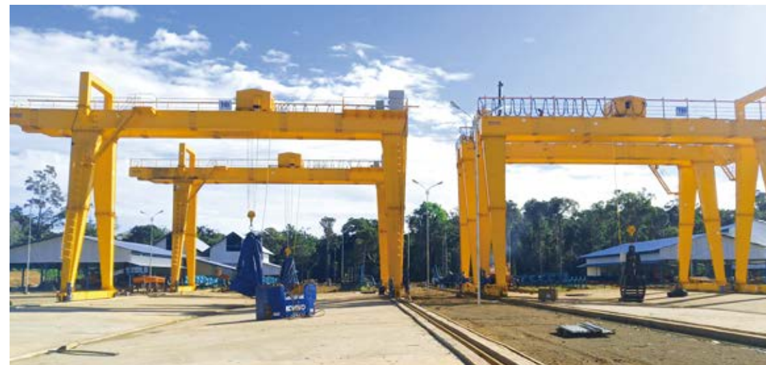
▲ MGZ16t Double Girder Grab Gantry Crane in Indonesia
