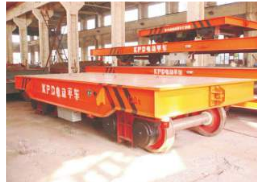
Rail Transfer Cart
